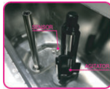
Agitator Operation Automatically Detect MIX OUT & MIX LOW by the sensor
