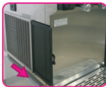
Pull out to remove the Air filter at the left side
