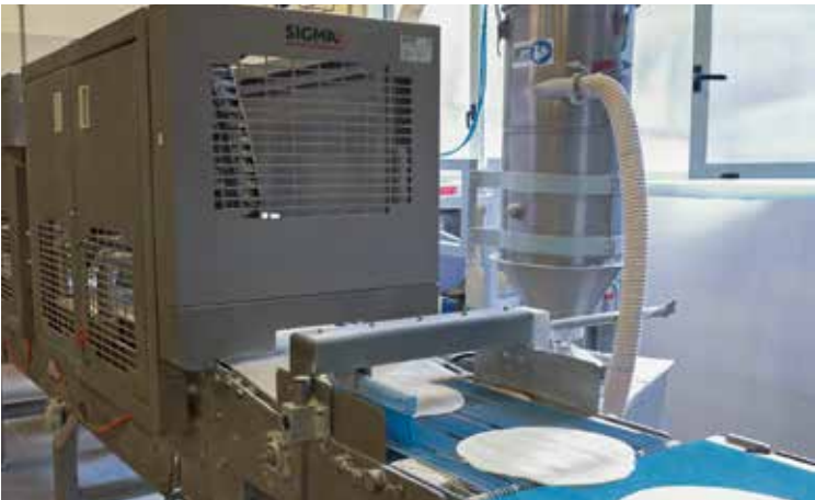
1 line with 2 spreading heads
