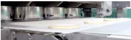
4 line with 8 spreading heads
