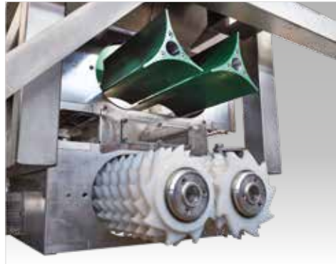
Feeding hopper with cutting group and crumbler
