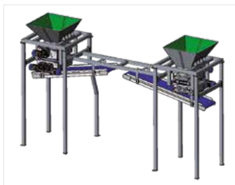
Multiple feeding hoppers with conveyor belts
