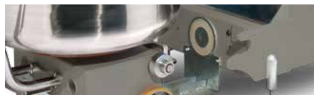
Bowl traction gear and electromagnetic hook for bowl trolley.
