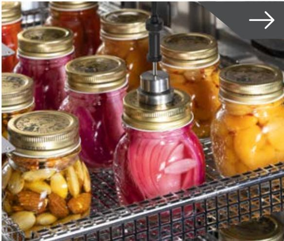
Thanks to the exclusive accessory for enabling **top quality, absolutely safe in-jar pasteurisation**, ACT.O actively controls the set thermal cycle, measuring the product's temperature directly in the heart of the jar, via the multipoint cooking probe. Any pasteurisation or jar-cooking process, even with large quantities, will be perfectly and completely controlled, exactly as you want it.
